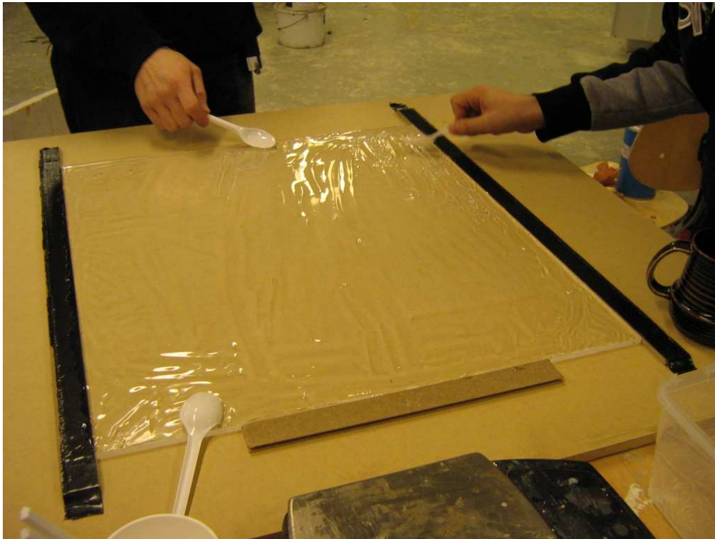
Image 30: Dividing the silicone rubber over the entire acrylic surface
